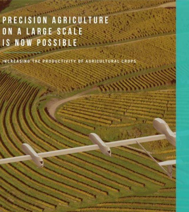
A SkyOrbiter is suitable for surveying vast rural areas and large-scale farms. The collected images have higher resolution than those obtained by conventional satellites, since this aerial platform is closer to the area being monitored.
