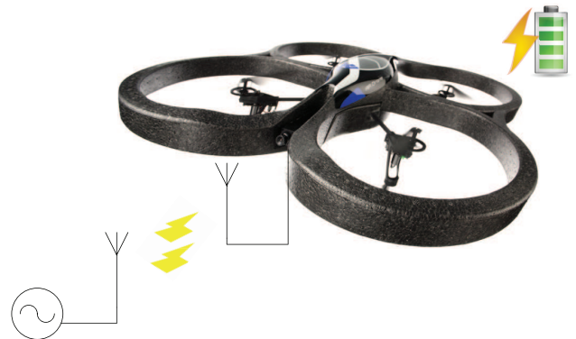
Fig. 2: Representation of a drone charging with resort to microwave power transmission.
