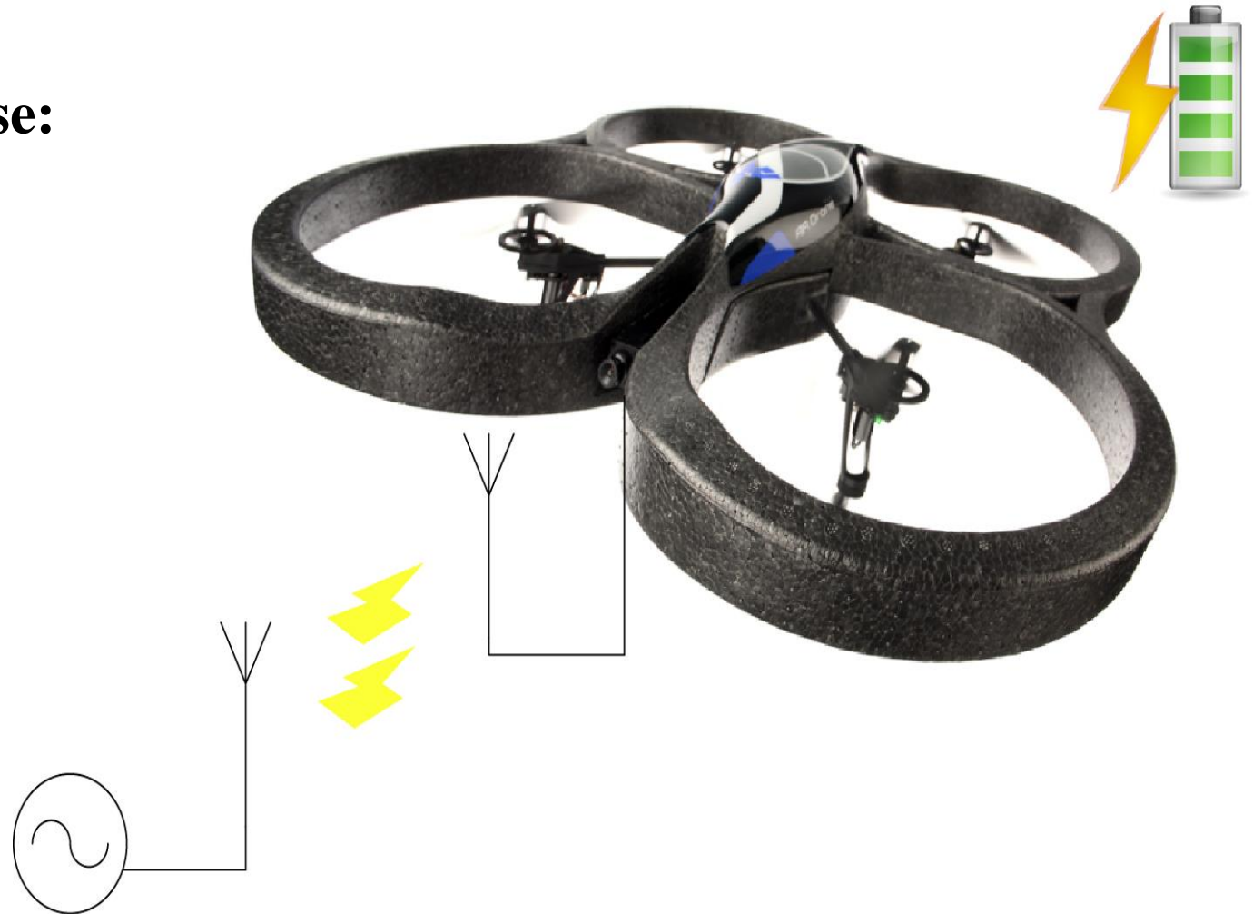
Fig. 2: Representation of a drone charging with resort to microwave power transmission.
