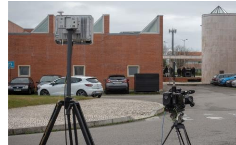
LSA controlled eNB and PMSE camera with a wireless data link
