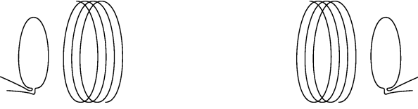
Fig. 1. Diagram of resonant magnetic coupling, composed by two single-turn coils and two high Q helical coils.
