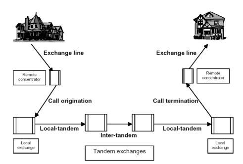
Figure 1: The fixed narrowband network
